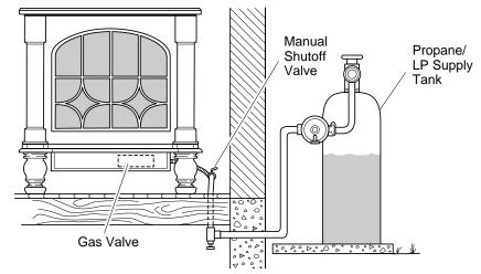
Figure 42 - Checking Gas Joints for Propane/LP Gas Burner System
